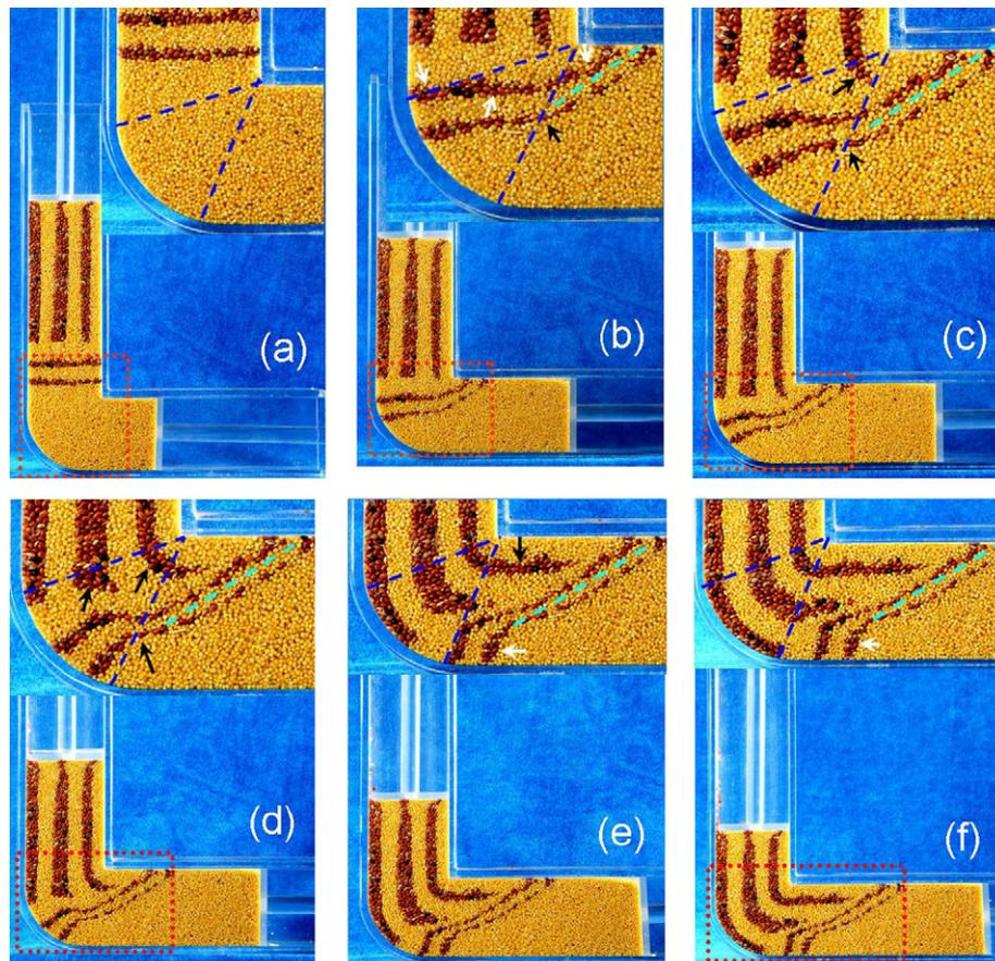
Fig. 2. In-situ observations of grain flow behavior in an ECAP die with  $\phi = 60^\circ$ .
