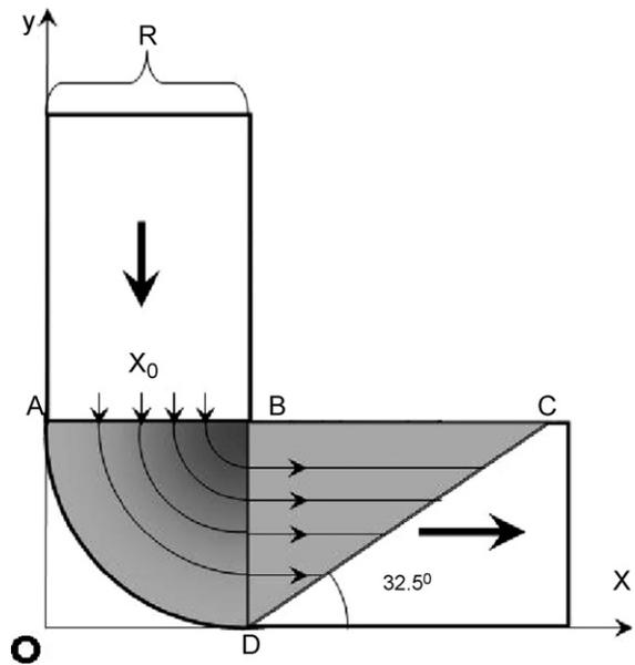
Fig. 5. Illustrations of the flow behavior in a round corner ECAP die.
