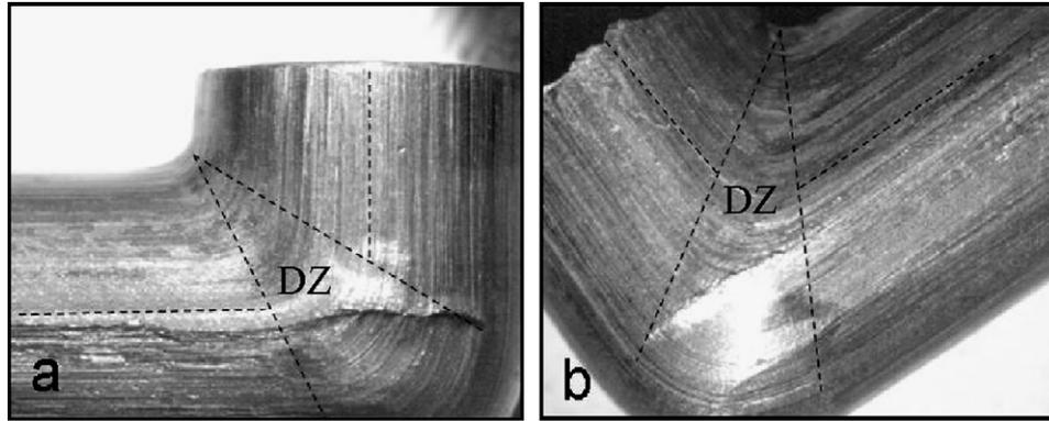
Fig. 3. Illustration of the flow traces on the surface of the real metals processed by ECAP. Figures (a) and (b) are viewed from two opposite directions in order to show the flow trace clearly.
