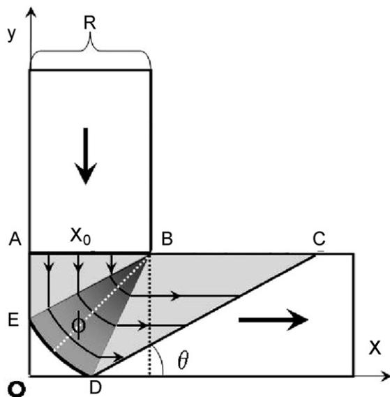
Fig. 4. Illustration of the flow behavior in an ECAP die with an arbitrary angle  $\phi$ .
