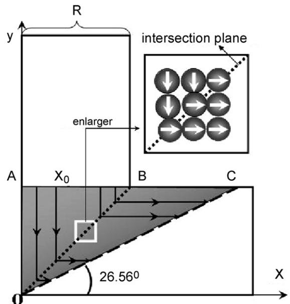
Fig. 6. Illustrations of the flow behavior in a right angle ECAP die.
