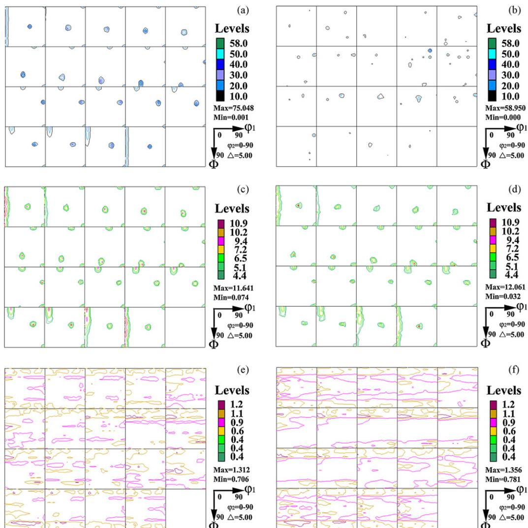
Fig. 2. Orientation distribution functions: (a) As-extruded 2009Al, (b) T4-treated extruded 2009Al, (c) as-extruded composite, (d) T4-treated extruded composite, (e) nugget zone of as-FSW composite and (f) nugget zone of T4-treated FSW composite.
