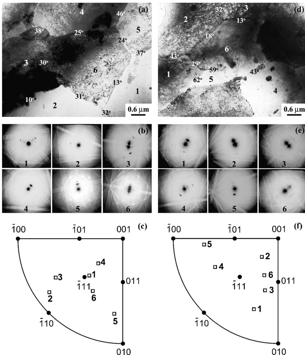
Fig. 1. Dynamically recrystallized grains with dominant HAGBs in NZ of FSW composites under (a) As-FSW condition and (d) T4-treatment condition: (b) and (e) Kikuchi's patterns for (a) and (d), (c) and (f) orientation relationship for neighboring grains in as-FSW and T4-treated composites, respectively.
