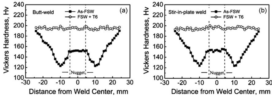
Fig. 5. Vickers hardness distribution of FSW 7075Al-T651 welds: (a) butt weld and (b) stir-in-plate weld (the advancing side is on the right).
