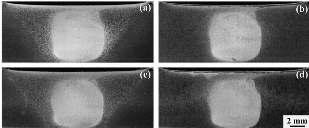
Fig. 1. Cross-sectional macrographs of FSW 7075Al-T651: (a) as-welded butt weld, (b) PW-T6 butt weld, (c) as-welded stir-in-plate weld, and (d) PW-T6 stir-in-plate weld (the advancing side is on the right).
