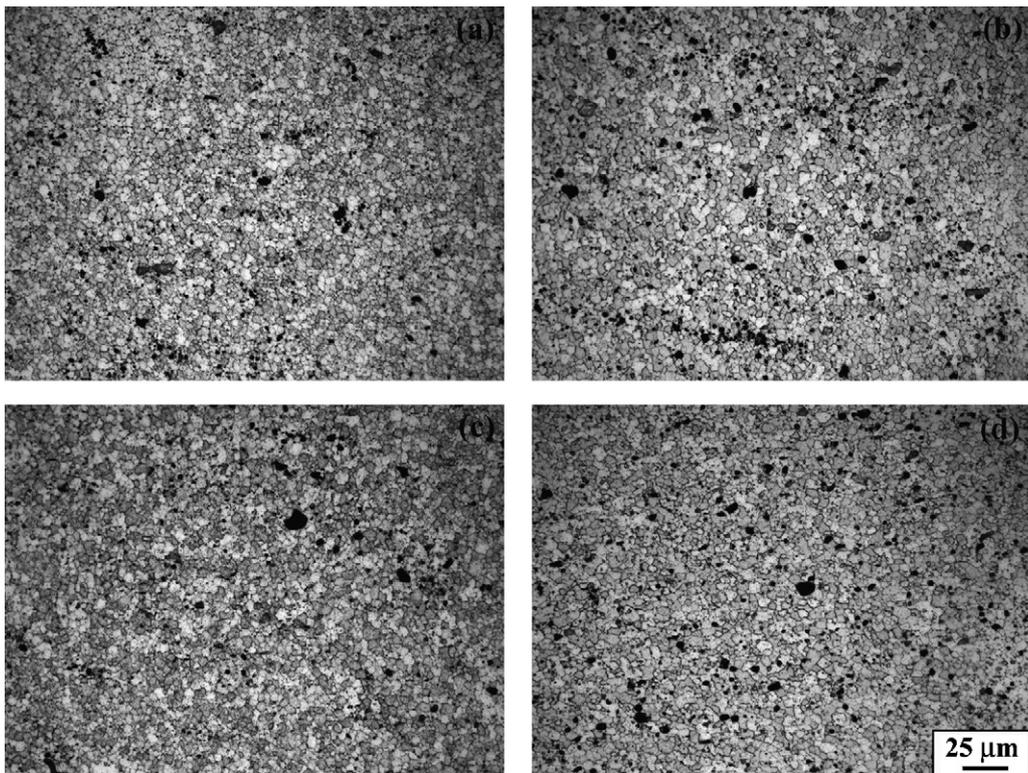
Fig. 2. Optical micrographs showing grain structure of the SZ in FSW 7075Al-T651: (a) as-welded butt weld, (b) PW-T6 butt weld, (c) as-welded stir-in-plate weld, and (d) PW-T6 stir-in-plate weld.
