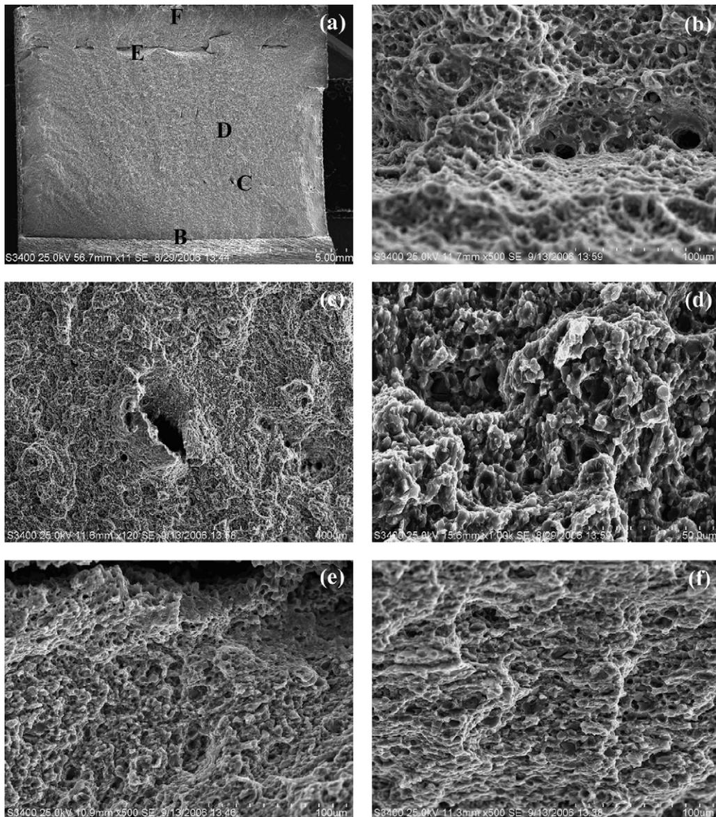
Fig. 8. SEM micrographs showing fracture surfaces of PW-T6 butt weld: (b)–(f) correspond to points B, C, D, E and F in (a), respectively.
