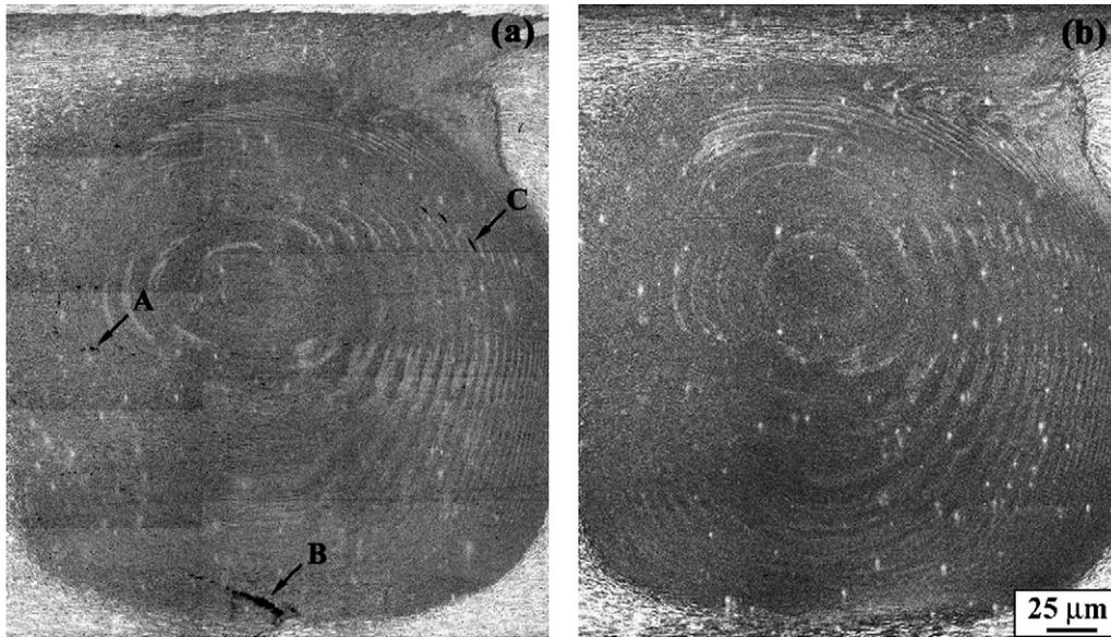
Fig. 3. Optical micrographs showing (a) zigzag micro-crack and discontinuous cavities on PW-T6 butt weld and (b) defect-free as-welded butt weld.
