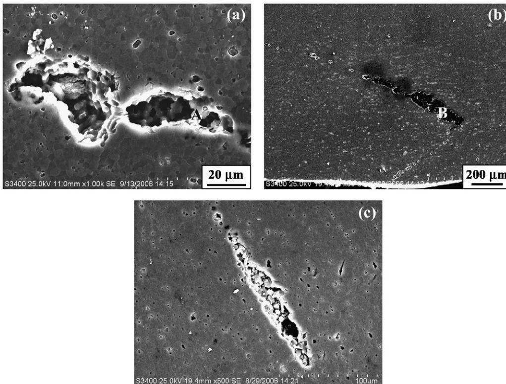
Fig. 4. SEM micrographs showing magnified view of PW-T6 butt weld: (a) cavity (point A in Fig. 3a), (b) zigzag micro-crack (point B in Fig. 3a), and (c) cavity along the onion ring (point C in Fig. 3a).
