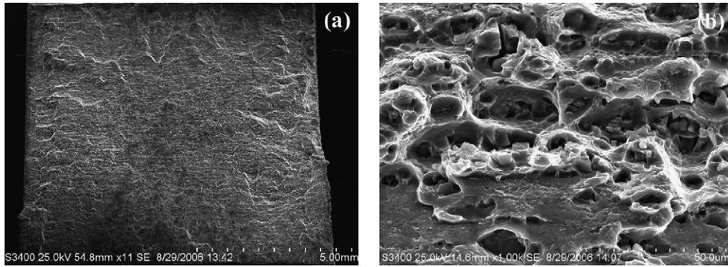
Fig. 7. SEM micrographs showing fracture surfaces of as-FSW butt weld.
