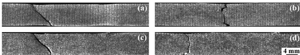
Fig. 6. Appearances of failed FSW joints: (a) as-welded butt weld, (b) PW-T6 butt weld, (c) as-welded stir-in-plate weld, and (d) PW-T6 stir-in-plate weld.
