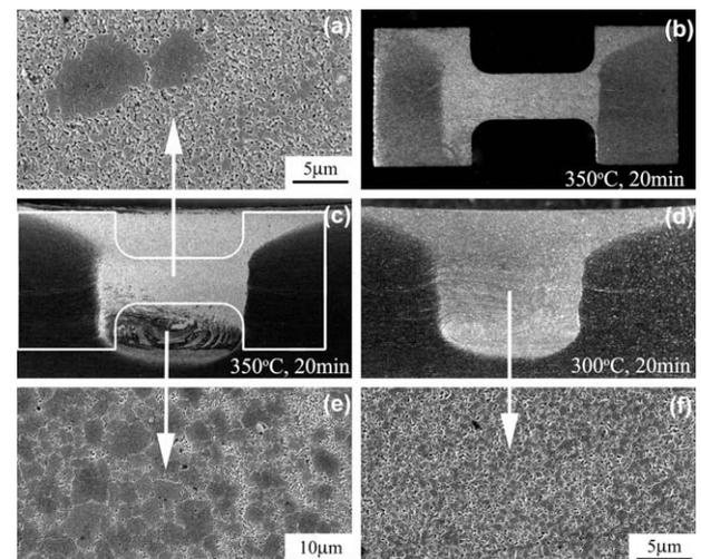
**Figure 4.** Microstructure evolution in FSP Al–Mg–Sc alloy annealed at different temperatures.
