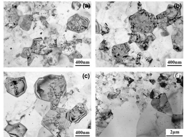
**Figure 3.** TEM microstructures of (a) as-FSP Al–Mg–Sc alloy and (b–d) FSP Al–Mg–Sc alloy annealed for 20 min at (b) 200 °C, (c) 300 °C and (d) 350 °C.
