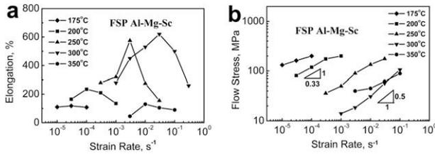
**Figure 2.** Variation of (a) elongation and (b) flow stress with initial strain rate for FSP Al–Mg–Sc alloy.
