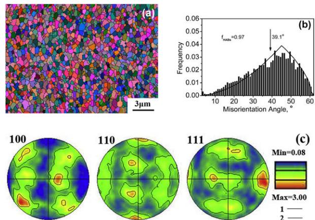
**Figure 1.** Microstructure of FSP Al–Mg–Sc alloy: (a) EBSD map, (b) boundary misorientation angle distribution, and (c) pole figures (sample surface was perpendicular to the FSP direction).
