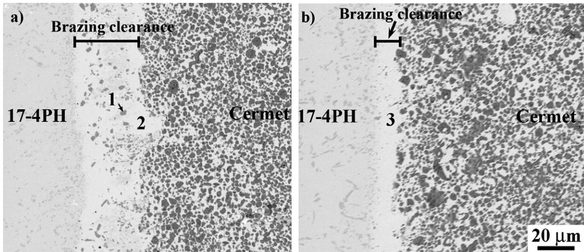
Fig. 2. Back-scattered electron images of joints brazed at (a) 1050 °C and (b) 1150 °C.
