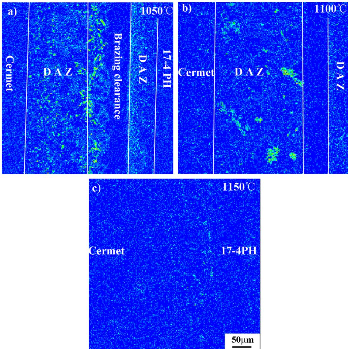
Fig. 3. Surface distribution of B in brazed joints of Ti(C,N)-based cermet and 17-4PH with BNi-2 at different brazing temperatures: (a) 1050 °C, (b) 1100 °C, and (c) 1150 °C.
