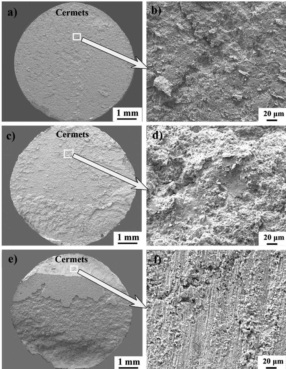
**Fig. 6.** Fractographs of brazed joints: (a and b) 1050 °C, (c and d) 1100 °C, and (e and f) 1150 °C.
