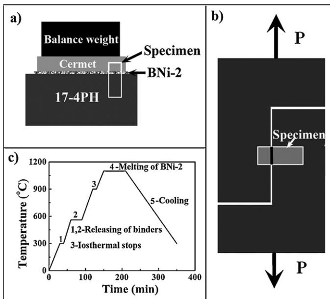
**Fig. 1.** Schematic illustration of (a) vacuum brazing, (b) fixtures for shear test, and (c) a thermal cycle of vacuum brazing.
