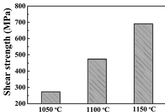
Fig. 5. Shear strength of Ti(C,N)-based cermet and 17-4PH joint vacuum brazed at different brazing temperatures with BNI-2.
