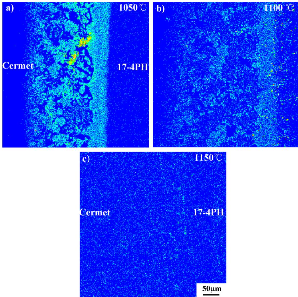
Fig. 4. Surface distribution of Si in brazed joints of Ti(C,N)-based cermet and 17-4PH with BNI-2 at different brazing temperatures: (a) 1050 °C, (b) 1100 °C, and (c) 1150 °C.
