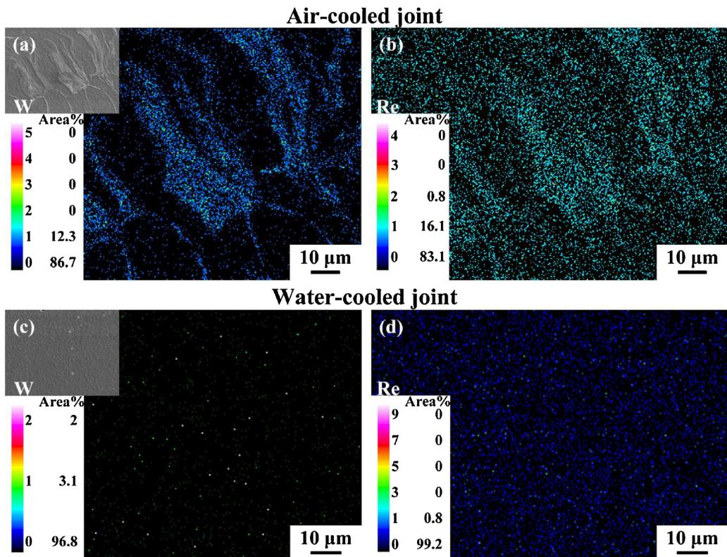
**Fig. 2.** W and Re distribution mapping of (a, b) air-cooled and (c, d) water-cooled FSW HNS joints.
