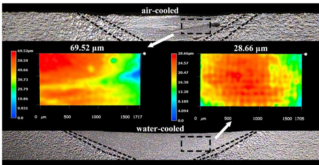
**Fig. 4.** Cross-sectional macrographs and 3D surface morphologies of FSW joints after immersion corrosion test.
