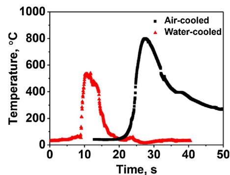
**Fig. 8.** Temperature histories during FSW of the bottom layer of workpiece close to welding tool pin.
