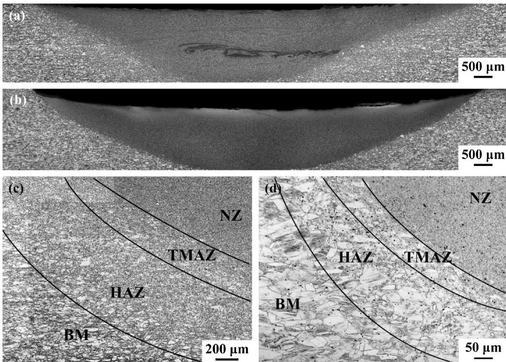
**Fig. 1.** Cross-sectional macrographs of (a) air-cooled and (b) water-cooled FSW HNS joints; detailed microstructures of (c) air-cooled and (d) water-cooled joints.
