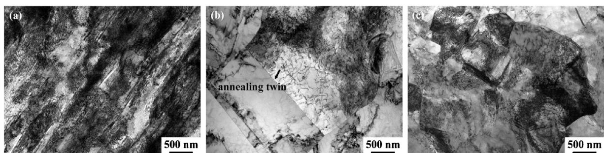
**Fig. 5.** Microstructure of (a) cold-rolled HNS, (b) HAZ of air-cooled joint, (c) HAZ of water-cooled joint.
