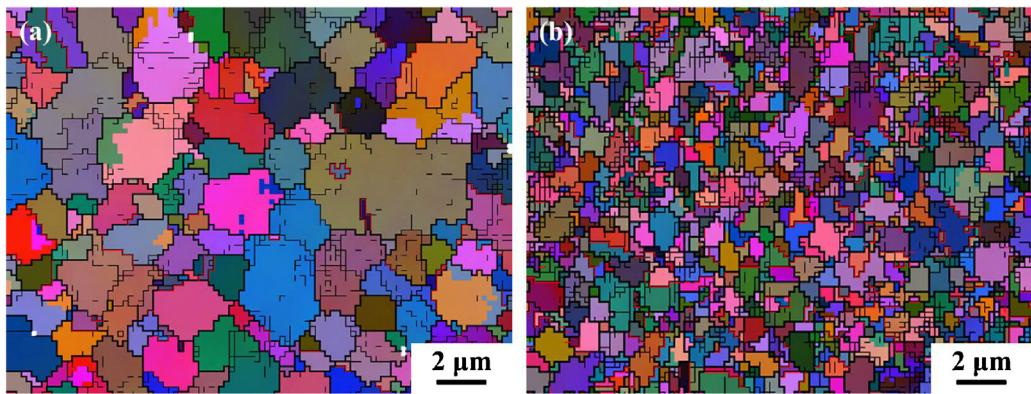
**Fig. 6.** EBSD maps of NZs of (a) air-cooled and (b) water-cooled joints.
