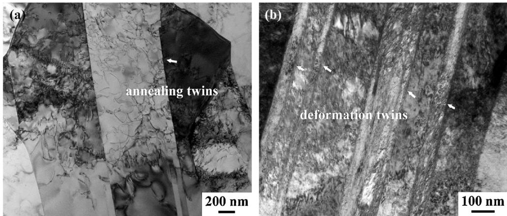
**Fig. 7.** Microstructure of NZs of (a) air-cooled and (b) water-cooled joints.
