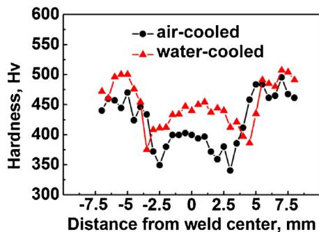
**Fig. 3.** Hardness profiles in cross-sections of FSW HNS joints.
