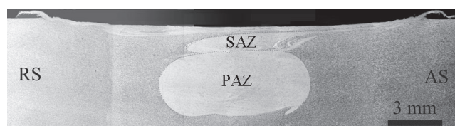
Fig. 2 Macrograph of single-pass FSP sample.
