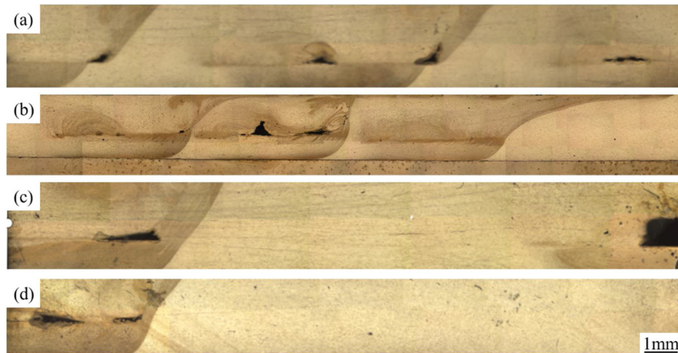
Fig. 9 – Microstructures of 1060Al/Q235 explosive composite plate after FSP with overlap (l/d): (a) 5/25; (b) 8/25; (c) 10/25 and (d) 15/25.
