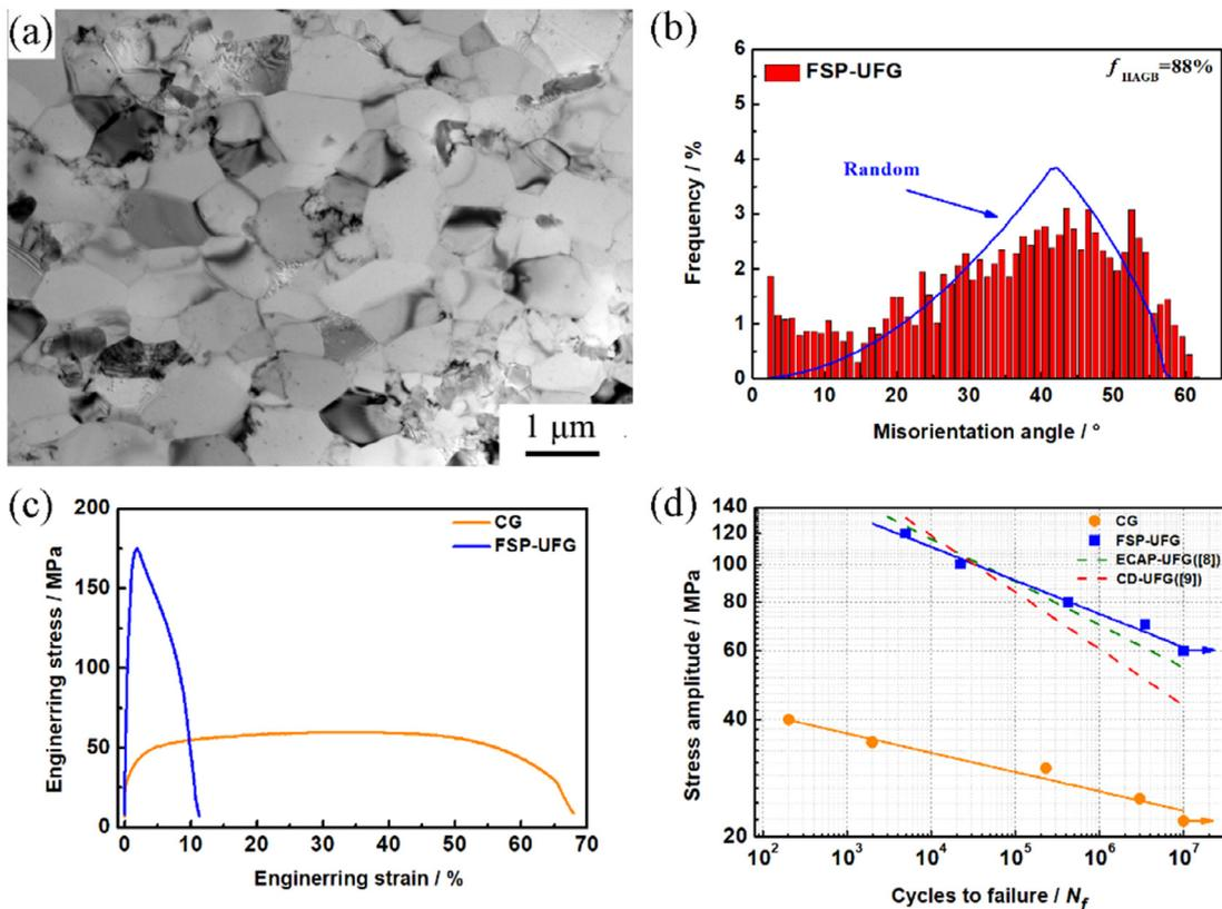
Fig. 1. (a) TEM microstructure, and (b) misorientation angle distribution of FSP-UFG Al, (c) tensile and (d) fatigue properties of CG and UFG samples [8,9]. CD-UFG: cold drawing UFG material. ECAP-UFG: UFG material fabricated by equal channel angle pressing.
