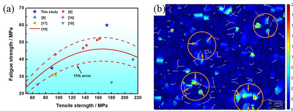
**Fig. 3.** (a) Relationship between fatigue strength and tensile strength in pure Al samples [8,9,16–19], (b) KAM analysis of FSP-UFG Al.
