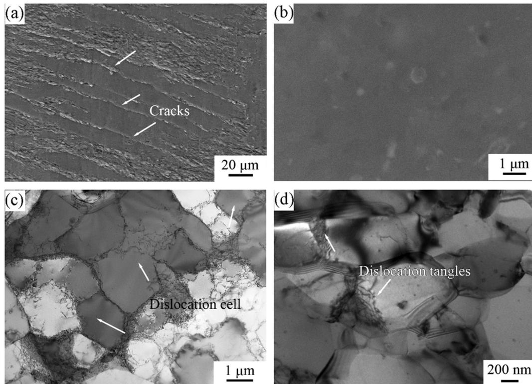
**Fig. 2.** Surface damage morphology and TEM microstructures after fatigue: (a) and (c) CG sample, (b) and (d) FSP-UFG sample.
