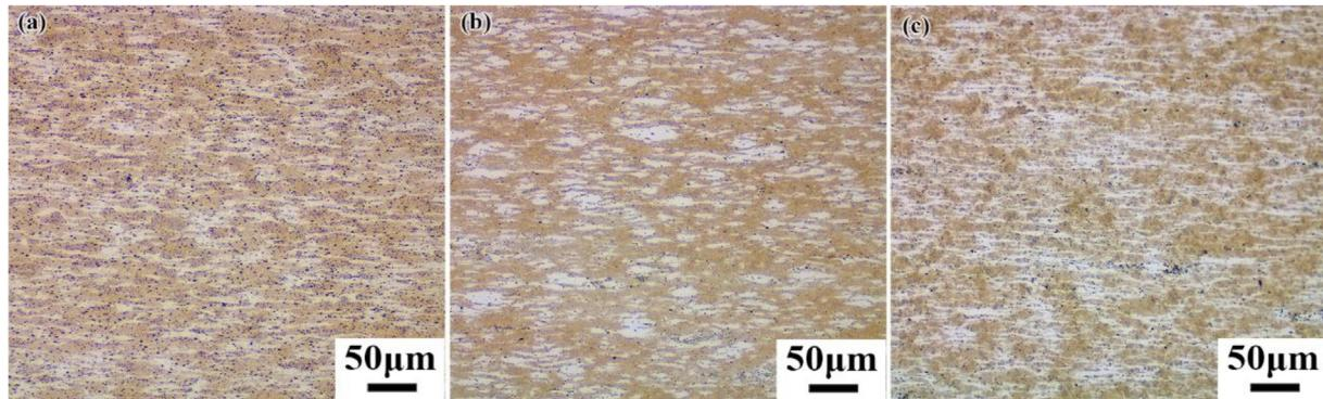
**Fig. 5.** OM images of bimodal CNT/2009Al composite specimens compressed to a true strain of 0.8 at (a) 300 °C with 1 s<sup>-1</sup>; (b) 450 °C with 1 s<sup>-1</sup> and (c) 450 °C with 0.001 s<sup>-1</sup>.
