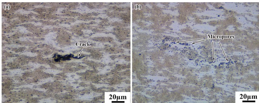
**Fig. 9.** The damage morphology of bimodal CNT/2009Al composite specimens compressed at (a) 300 °C with 1 s<sup>-1</sup>, (b) 450 °C with 0.001 s<sup>-1</sup>.
