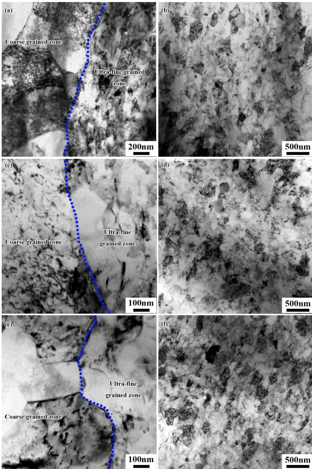
**Fig. 8.** TEM images of bimodal CNT/2009Al composite specimens compressed to a true strain of 0.8 at (a), (b) 350 °C with 1 s<sup>-1</sup>, (c) (d) 450 °C with 1 s<sup>-1</sup>, (e) (f) 450 °C with 0.001 s<sup>-1</sup>.
