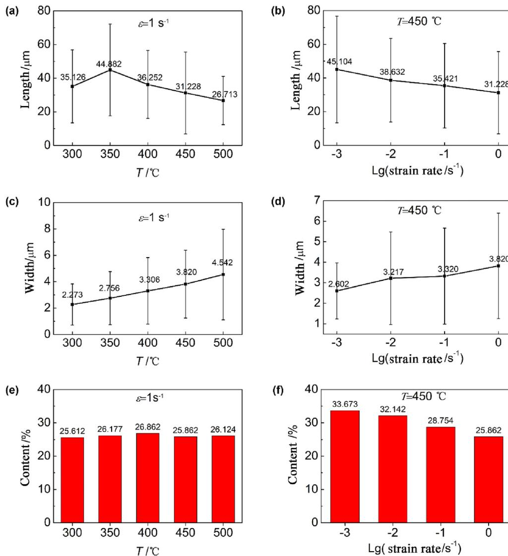
**Fig. 6.** The statistical results of (a), (c), (e) average length, width and content of coarse grained zones at strain of 1 s<sup>-1</sup> with different temperatures; (b), (d), (f) average length, width and content of coarse grained zones at temperature of 450 °C with different strain rates.
