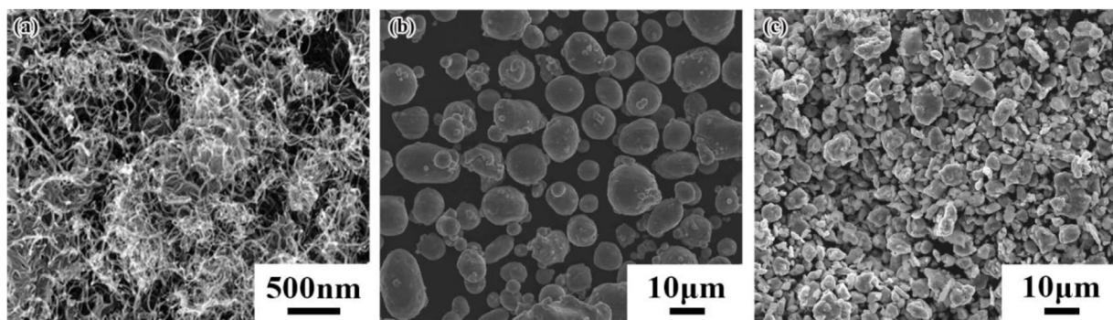
**Fig. 1.** Powder morphologies of (a) the raw CNTs, (b) the raw 2009Al alloy, (c) the ball-milled CNT/2009Al.
