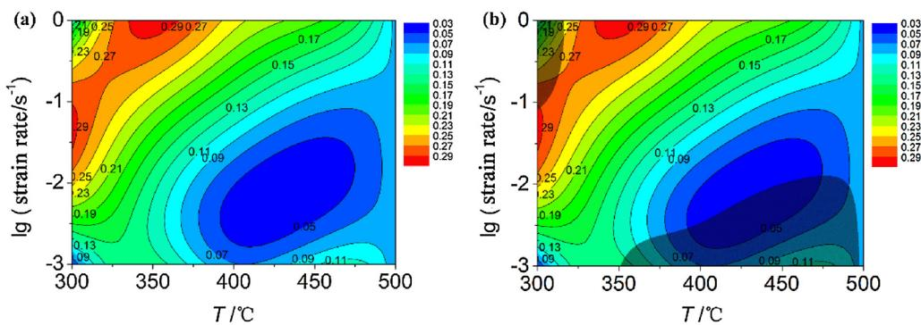
**Fig. 4.** Processing maps of bimodal CNT/2009Al composite: (a) power dissipation map; (b) processing map containing instable zone.
