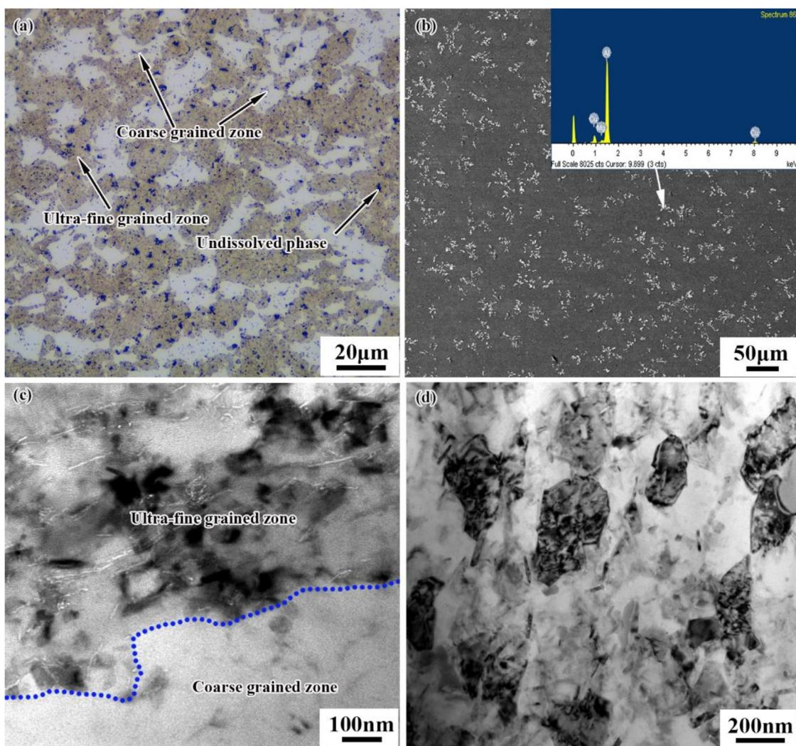
**Fig. 2.** Initial microstructures of as hot-pressed CNT/2009Al composite: (a) OM image of macrostructure, (b) SEM back-scattered electron image and EDS of undissolved phases, (c) TEM image of CNT distribution, and (d) TEM image of grain structure in ultra-fine grain zones.
