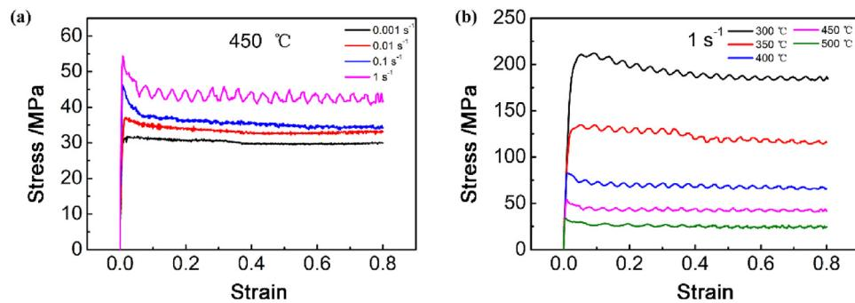
**Fig. 3.** Compressive true stress-true strain curves of bimodal CNT/2009Al composite specimens at (a) 450 °C with different strain rates; (b) 1 s<sup>-1</sup> with different temperatures.
