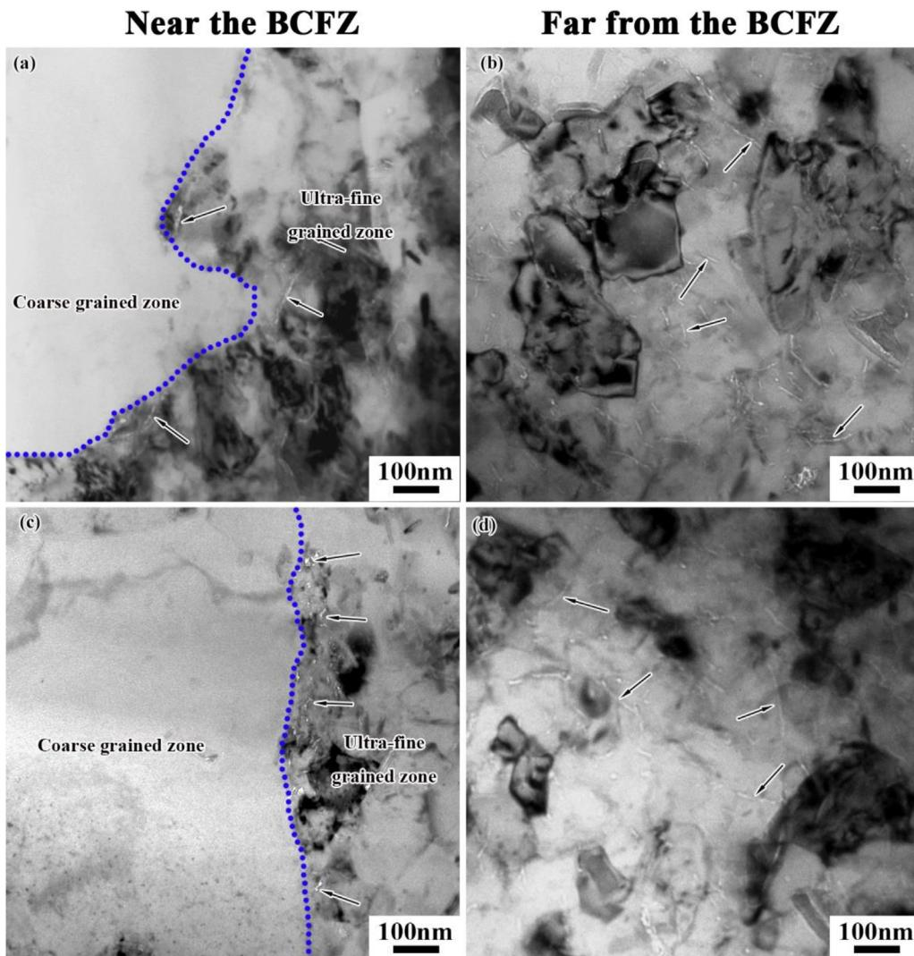
**Fig. 10.** The CNT distribution for the specimens compressed to a true strain of 0.8 at (a), (b) 300 °C with 1 s<sup>-1</sup>, (c) (d) 450 °C with 0.001 s<sup>-1</sup>.
