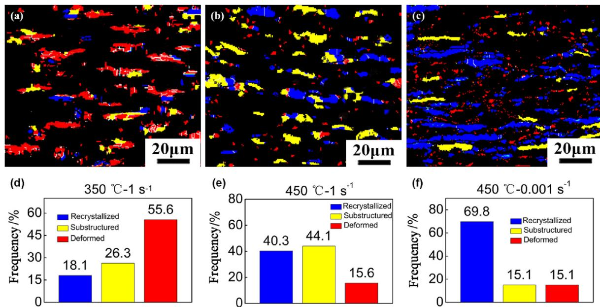
**Fig. 7.** Grain type distribution maps characterized by EBSD and their proportions in coarse grained zones compressed at (a), (d) 350 °C with 1 s<sup>-1</sup>, (b) (e) 450 °C with 1 s<sup>-1</sup>, (c) (f) 450 °C with 0.001 s<sup>-1</sup>.
