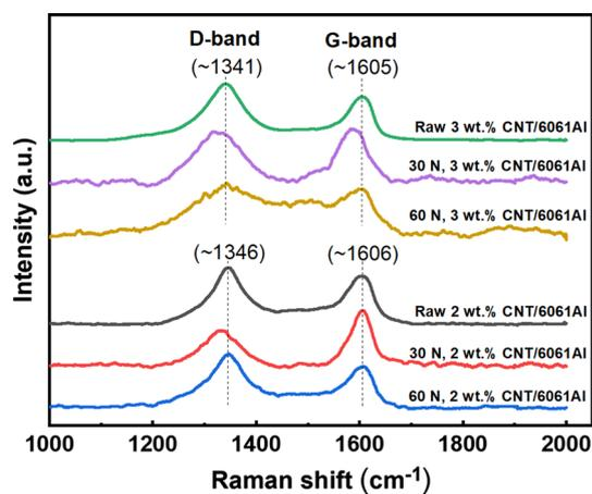
Fig. 16 Raman spectra of the wear surfaces of 2 wt% and 3 wt% CNT/6061Al composites under 30 N and 60 N
