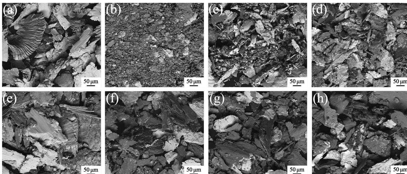
**Fig. 10** SEM images showing the wear debris morphology of the CNT/6061Al composites with different CNT concentrations under 30 N: **a** 0 wt%; **b** 1 wt%; **c** 2 wt%; **d** 3 wt%; 60 N: **e** 0 wt%; **f** 1 wt%; **g** 2 wt%; **h** 3 wt%
