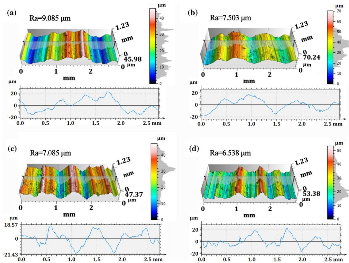
**Fig. 12** 3d profilogram of wear tracks for the CNT/6061Al composites with different CNT concentrations under 60 N: **a** matrix alloy; **b** 1 wt%; **c** 2 wt%; **d** 3 wt%
