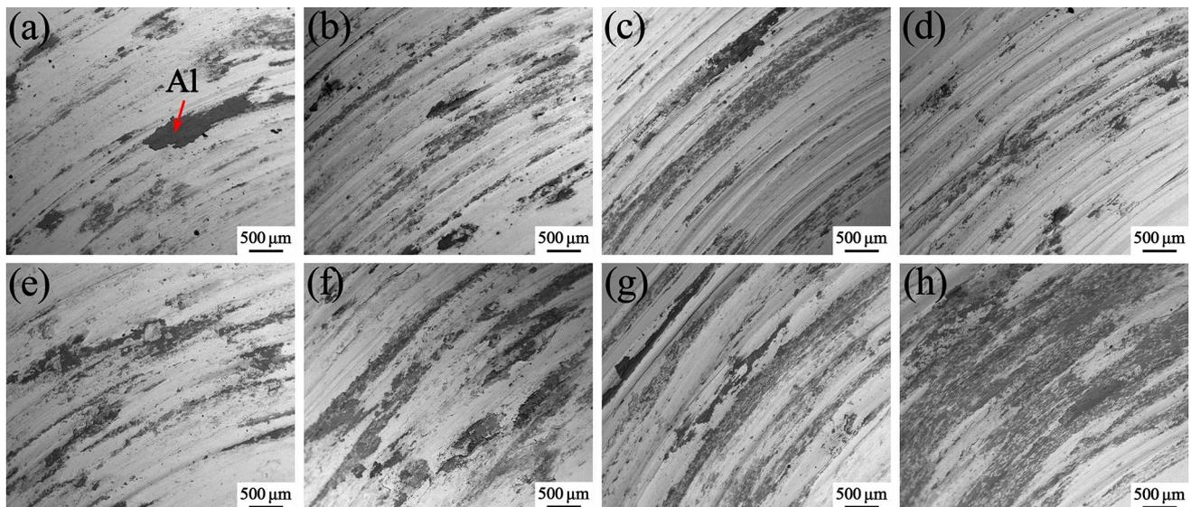
**Fig. 9** SEM images showing the wear surface morphology of counterparts for CNT/6061Al composites with different CNT concentrations under 30 N: **a** 0 wt%, **b** 1 wt%, **c** 2 wt%, **d** 3 wt%, 60 N: **e** 0 wt%, **f** 1 wt%, **g** 2 wt%, **h** 3 wt%
