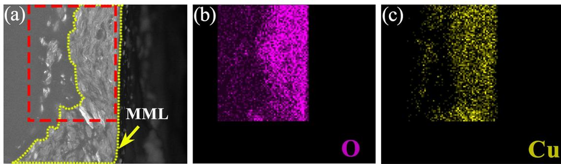
Fig. 14 EDS analysis of the typical MML for the 2 wt% CNT/6061Al composite
