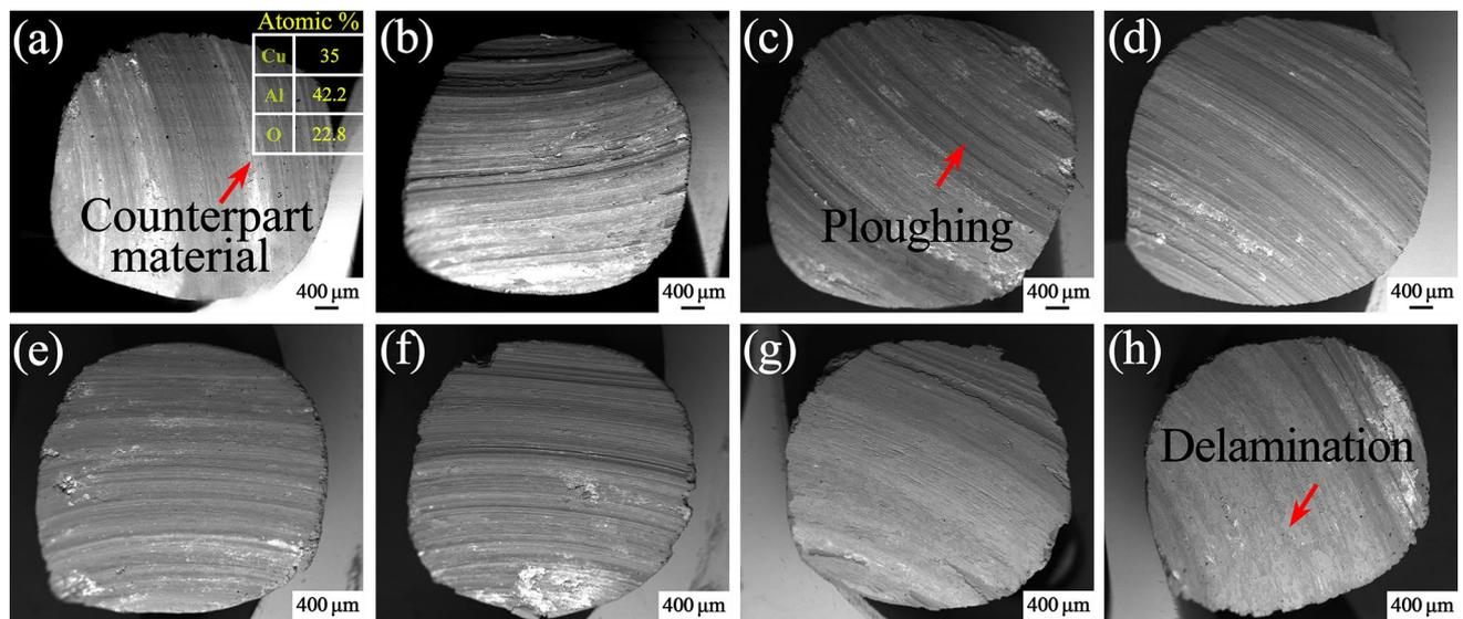
**Fig. 6** SEM images showing the wear surface morphology of CNT/6061Al composites with different CNT concentrations under 30 N: a 0 wt%, b 1 wt%, c 2 wt%, d 3 wt%, 60 N: e 0 wt%, f 1 wt%, g 2 wt%, h 3 wt%
