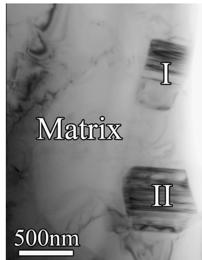
Fig. 1. Bright-field TEM image showing the precipitations of M_2B -type boride within the matrix ( \gamma/\gamma' ). Note that the precipitations feature highly dense stacking faults.
