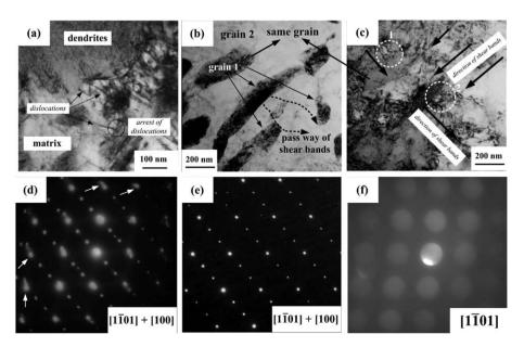
Fig. 7. TEM bright-field images (a-c), the corresponding selected area diffraction patterns (d and e) and a microbeam diffraction pattern (f) of the nanostructured matrix of the partially (a and d) and fully deformed samples (b, c, e, and f).
