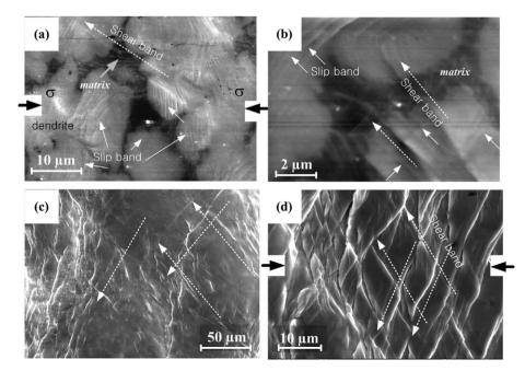
Fig. 3. SEM secondary electron images obtained from the surfaces of the partially deformed (a and b) and fully deformed (c and d) samples.
