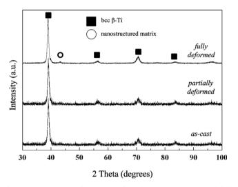
Fig. 2. XRD patterns of as-cast, partially deformed ( $\epsilon_p = 8\%$ ) and fully deformed ( $\epsilon_p = 25\%$ ) samples.
