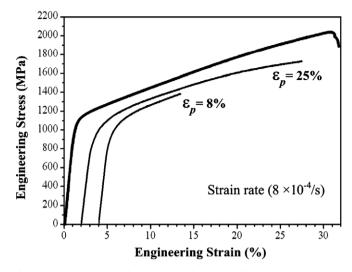
Fig. 1. Typical compressive stress–strain curves of the  $Ti_{66.1}Nb_{13.9}Ni_{4.8}$ -Cu\_8Sn<sub>7.2</sub> nanostructure–dendrite composite. The tests were stopped at different strains ( $\epsilon_p=8\%$  and 25%) for SEM and TEM observation.
