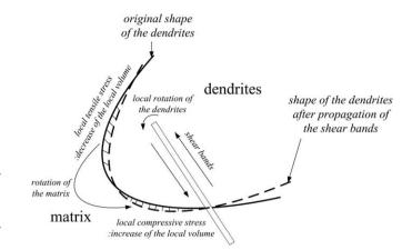
Fig. 9. Schematic of the local volume changes at the interfaces between the dendrites and the nanostructured matrix, and of the rotation of the nanostructured matrix.
