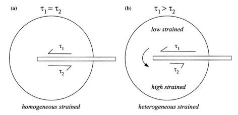
Fig. 8. Schematics to explain the rotation of the dendrites using the imbalance of the shear stress.
