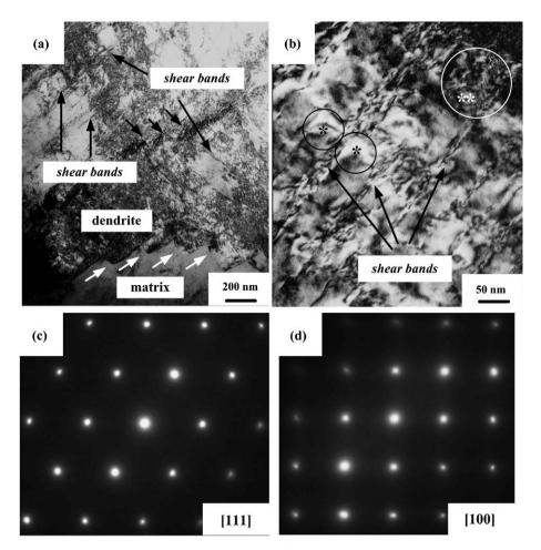
Fig. 5. TEM bright-field images (a and b) and the corresponding selected area diffraction patterns (c and d) of the dendrites of the fully deformed sample.
