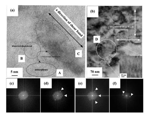
Fig. 6. HRTEM images (a and b) and the Fourier transformed patterns (c-f) from a dendrite of the fully deformed sample.
