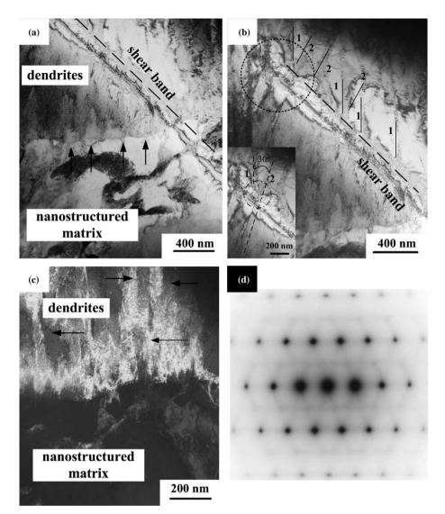
Fig. 4. TEM bright-field images (a and b), dark-field image (c) and the corresponding selected area diffraction pattern (d) of the dendrites of the partially deformed sample.
