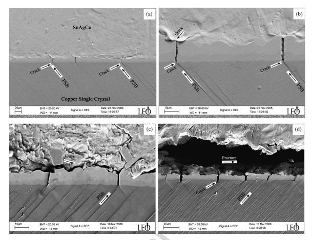
Fig. 5. SEM micrographs of the damage processes at the aged SnAgCu/copper single crystal interface during cyclic deformation: (a) 200 cycles, (b) 200 cycles, the magnified image of (a), (c) 2000 cycles, and (d) 3000 cycles.
