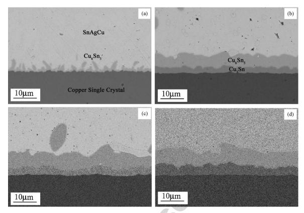
Fig. 2. SEM-backscattered electron micrographs of the morphology of IMCs at the SnAgCu/copper single crystal interface: (a) as-reflowed, (b) aged at 170 °C for 4 days, (c) 7 days, and (d) 16 days.
