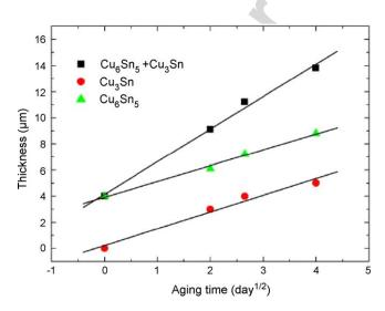
Fig. 3. Dependence of the thicknesses for the IMC layers at the SnAgCu/copper single crystal joint on the aging time at 170 °C.
