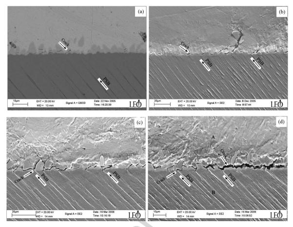
Fig. 4. SEM micrographs of the damage processes at the as-reflowed SnAgCu/copper single crystal interface during cyclic deformation: (a) 650 cycles, (b) 3000 cycles, (c) and (d) 4000 cycles.
