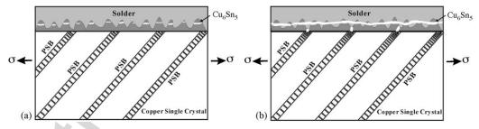
Fig. 7. Illustration of the damage process at the as-reflowed interface under the interaction of PSBs with the interface: (a) fracture of the protrudes of IMC and (b) cracking at the intersection site of PSBs with the interface and failure along the interface of solder/IMC layer.
