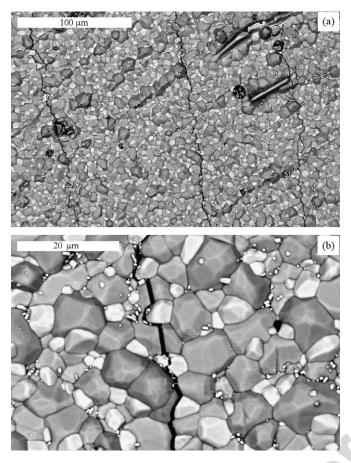
Fig. 6. SEM-second electron micrographs of the crack propagation within the  $Cu_6Sn_5$  IMC layer: (a) straight propagation path and (b) intergranular and transgranular manners.
