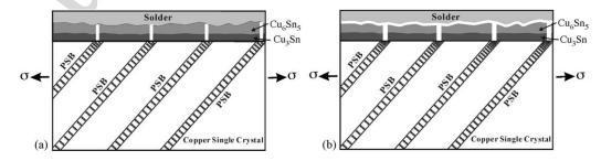
Fig. 8. Illustration of the damage process at the aged interface under the interaction of PSBs with the interface: (a) cracking at the intersection site of PSBs with the interface and (b) failure along the interface of solder/IMC layer.
