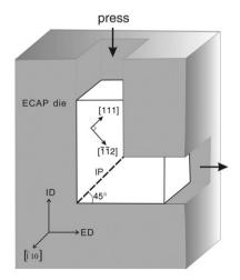
Figure 1. Schematic illustration of the ECAP coordinates and current experimental design (ID for insert direction and ED for extrusion direction).
