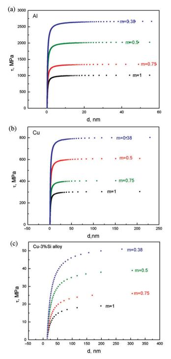
Figure 13. Plot for the variation in critical shear stress for propagating Shockley partials with the shear factor value for (a) Al, (b) Cu and (c) Cu-3% Si alloy.
