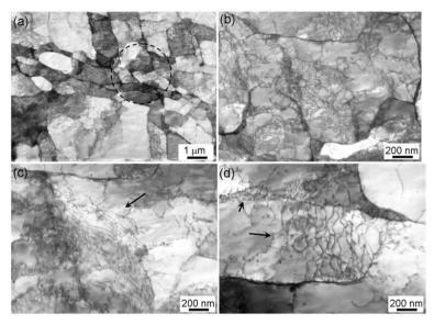
Figure 4. TEM micrographs of the dislocation configurations at the side of a shear band. (a) Low magnification morphology and (b)–(d) high magnification dislocation patterns.
