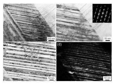
Figure 10. TEM micrographs of the deformation twins formed in the deformed Cu-3% Si alloy. (a) Low magnification image, (b) high magnification image at boundary of the band, (c) high magnification image in the inner part and (d) the corresponding dark-field image.
