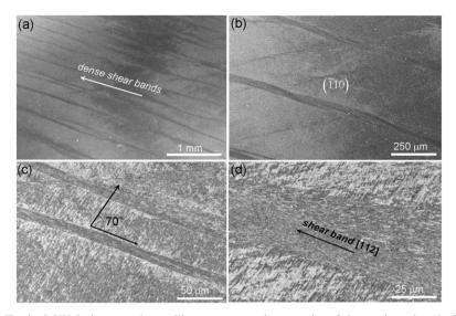
Figure 5. Typical SEM electron channelling contrast micrographs of dense shear bands formed on the ID–ED plane of a Cu single crystal during the ECAP process. (a) Macroscopic SEM image and (b)–(d) magnified SEM images.
