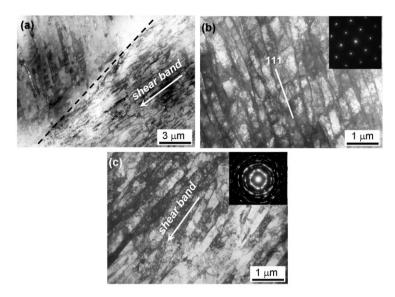
Figure 6. TEM micrographs of the deformation microstructures for a Cu crystal. (a) Image of the interface between matrix and shear band, (b) dense dislocation walls formed in the matrix region and (c) fine strip structures in the shear band.
