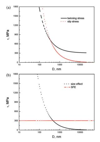
Figure 14. Plot of (a) variation in twinning stress and slip stress with grain size, (b) contribution of SFE (Equation (13)) and size effect (Equation (14)) to twinning stress with varying length-scale.
