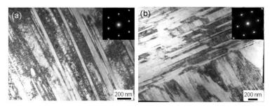
Figure 8. TEM micrographs of the planar slip features in the Cu-3% Si alloy after single-pass ECAP. (a) one direction of planar slip; (b) two directions of planar slip.
