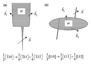
Figure 11. Schematic illustration of the dislocation reaction for nucleating partials. (a) Perfect dislocation dissociated into two Shockley partials and (b) perfect dislocation dissociated into a Frank and a Shockley partial.
