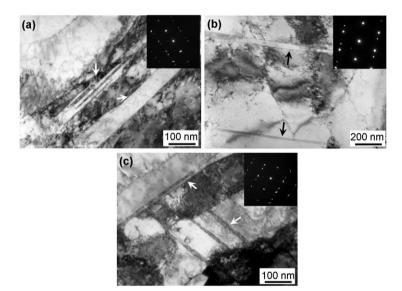
Figure 7. TEM micrographs of (a) Type I, (b) Type II and (c) Type III deformation twins formed in a Cu single crystal.
