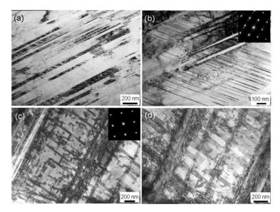
Figure 9. TEM micrographs of the numerous twins and SFs formed within the narrow banding structures in the Cu-3% Si alloy. (a, b) Fine twins and SFs in the banding structures and (c, d) images of SFs viewed from the [001] direction.
