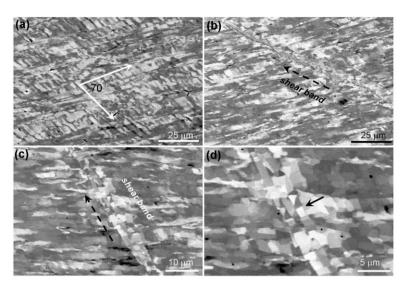
Figure 2. Typical SEM electron channelling contrast micrographs of deformation microstructures of an Al single crystal after single-pass ECAP. (a) Coarse ribbon structures and (b)–(d) shear bands formed during extrusion.
