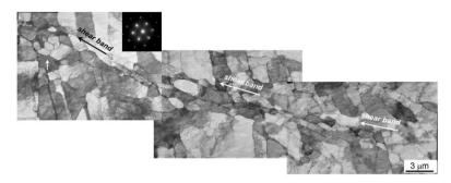
Figure 3. TEM micrographs of a narrow shear band formed in an Al single crystal during extrusion.
